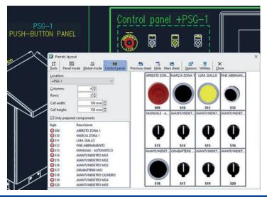
by dragging and dropping on a user-definable grid, with identification symbols for the type of components used.
