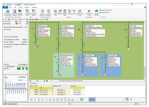
Ampère Evolution is the software for calculating extended electricity networks, with distributed generation from RES, wind and photovoltaic sources. Calculates LV and MV networks, alternating and direct, according to CEI 64-8, 11-17, 11-25, 17-1, CEI EN 62271-100, IEC 60364, 60909, 61660-1, 61936-1 and international standard NF C 15-100 (French), UNE 20460 (Spanish), BS 7671 (English), NBR 5410 (Brazilian), NFPA 70: NEC (American).
